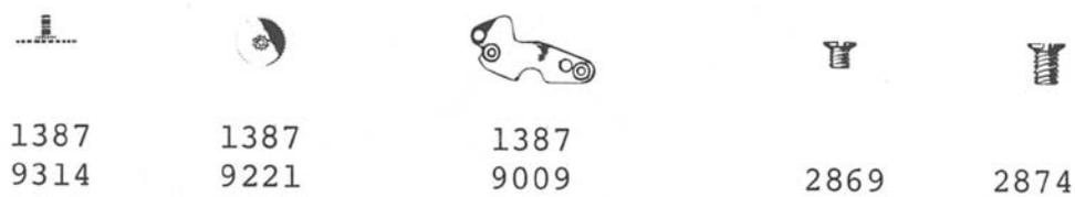
**Remark** The short screw 2869 of the minute wheel train bridge should be screwed close to the corrector.
